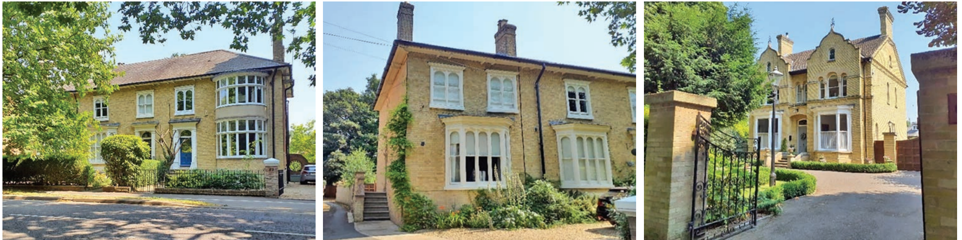
Elaborate early 20th century detailing, including iron balconies and railing, prominent curved bay windows and Dutch gables
